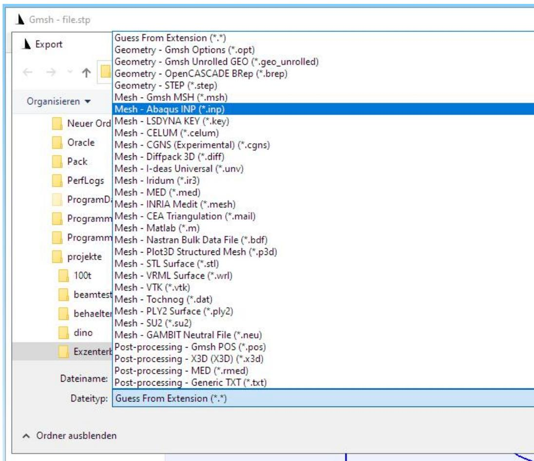
After the GMSH export, select "Generate Surface Model" to be able to select the 8 main surfaces of the eccentric bolt for the surface load and clamping.
