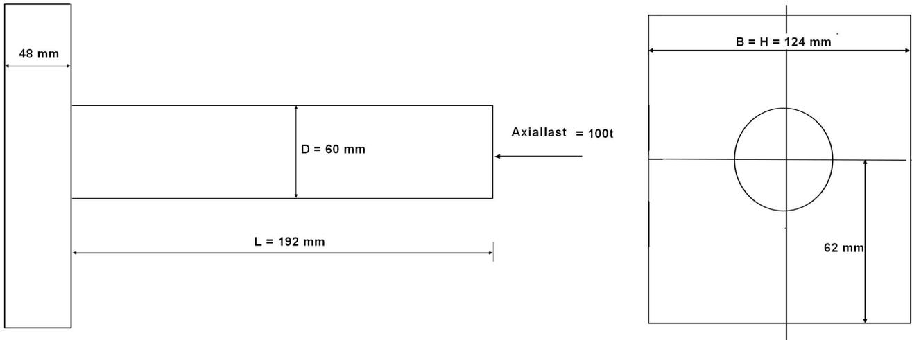
$$\begin{aligned} \text{Axial Stress} &= F_A / A_Z = 1\,000\,000 \text{ N} / 3.1416 \cdot D^2 / 4 \\ &= 1\,000\,000 \text{ N} \cdot 4 / 3.1416 \cdot 60^2 \text{ mm}^2 = 353.7 \text{ N/mm}^2 \end{aligned}$$
