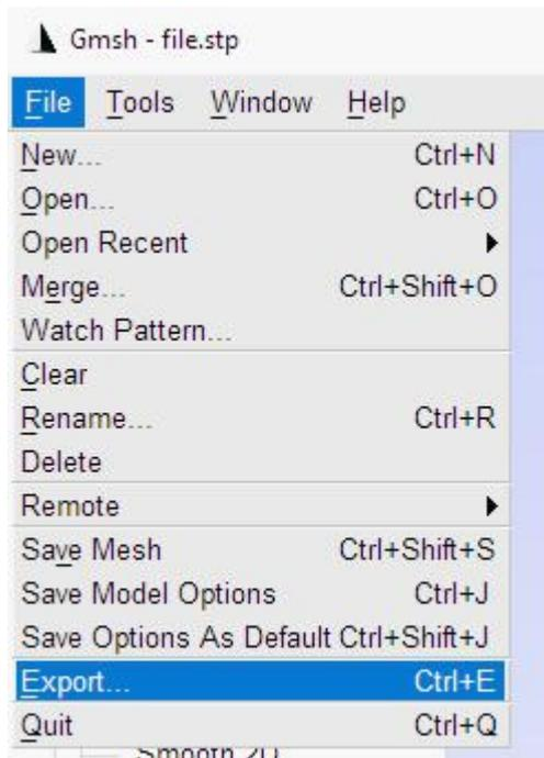
If the mesh is saved in the same directory with the name "file", it is automatically imported and displayed by MEANS V12.
